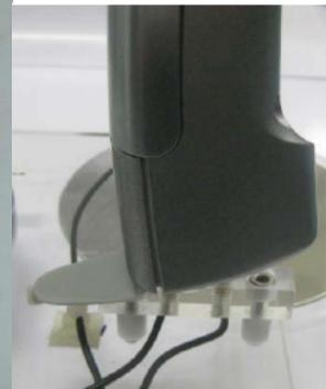
Note: Open the rubber cover, and insert two connector contacts. The hand grips direction like photograph.
